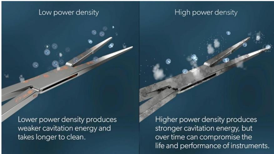
What is the effect of differences in power density? We will use the same frequency so the bubbles will be the same size. Now we can compare the differences in power density.
