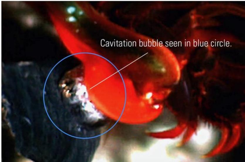
Cavitation is the energy process of cleaning instruments during ultrasonic cleaning. Ultrasonic cavitation begins with sound at a very high pitch or frequency. Breaking down the meaning of ultrasonic you have ultra, meaning extremely, and sonic meaning sound, where ultra refers to extremely high sound frequency. It is the very high frequency of sound vibrations in water that cavitation can occur.
